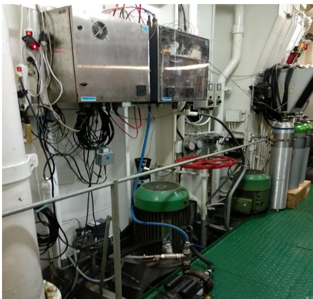
Equipment for carbon dioxide measurements in the RENATE P vessel used by ULPGC. The vessel travels biweekly from the Canary Islands to Barcelona. Photo by Melchor González Dávila.
