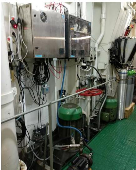
*Equipment for carbon dioxide measurements in the RENATE P vessel used by ULPGC. The vessel travels biweekly from the Canary Islands to Barcelona. Photo by Melchor González Dávila.*
